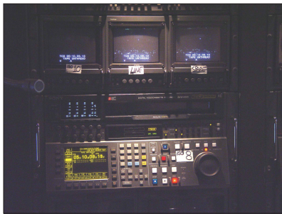
Figure 5.21 A mainstay on trucks today is the Sony DVW-A500 Digital Betacam. The "A" in the designation means that this digital VTR can play back analog Betacam tapes, even though the two formats are physically quite different. It's able to do this through DT head and TBC magic. The Digital Betacam uses a mild 2:1 JPEG compression. It records 10-bit component video and 20-bit AES audio sampled at 48KHz. The bit rate onto tape is 127.8Mb/s. The evolution from tape to server now taking place in the tape compartments of most production trucks is also happening inside the VTR. Sony introduced the hybrid VTR with their SK series. A hybrid VTR is a VTR with an internal disk drive. This would allow one VTR to edit or assemble raw footage onto its internal disk drive by itself, without using a second VTR.
