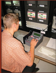
Figure 5.26 Controller for multichannel server. One operator can control many channels of video and audio.
