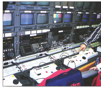
Figure 5.22 This HD truck's tape compartment includes Sony HDCam high-definition VTRs, with a standard-definition Sony DVW-A500 in the center. The HDCam subsamples video at 3:1:1 at eight bits, so as not to have to compress the resulting data as much. The data rate onto tape is 140Mb/s. (Source: Tim Stoffel)
