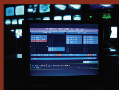
Figure 5.27 The GUI that a server operator uses to manage clips that have been saved and will be used later, either separately or as part of a highlight package.
